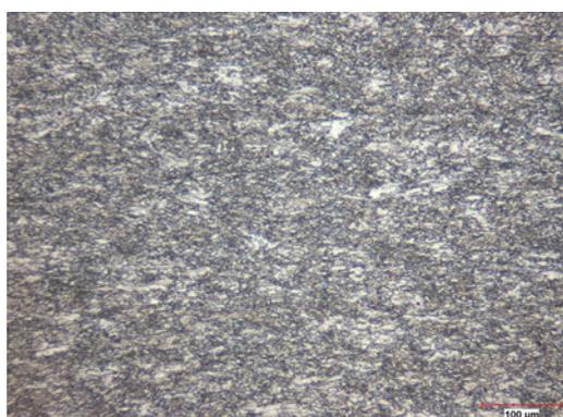
Figure 3. Microstructure of X70-1 (X100)
