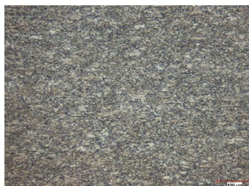
Figure 4. Microstructure of X70-2 (X100)
