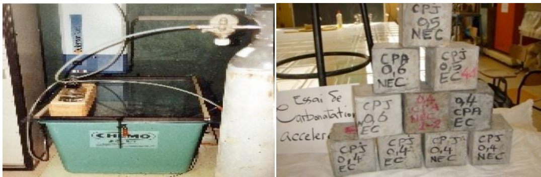
Figure 2: (a) Accelerated carbonation chamber; (a) Specimens in the carbonation chamber under accelerated conditions
