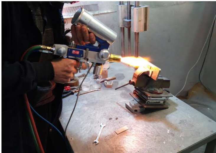
Fig. 4. Coating of Ti substrate by HVOF method
