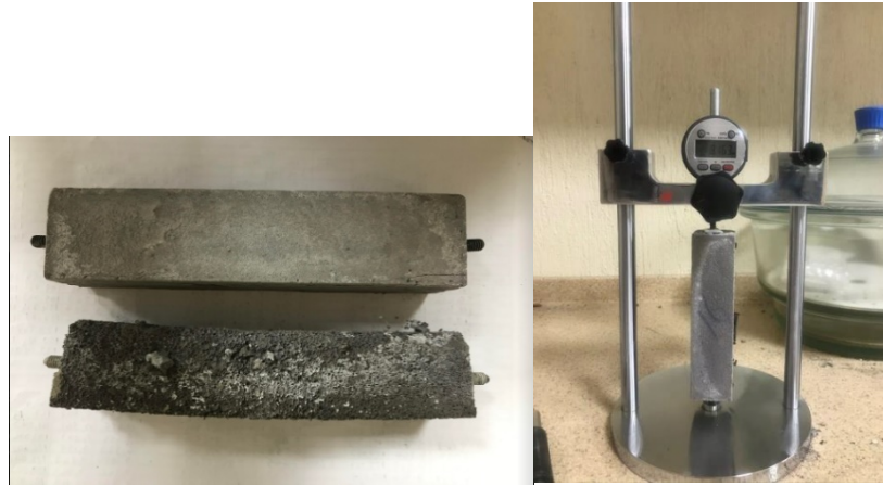
Figure 2.a) Drying shrinkage samples, and b) analysis equipment.
