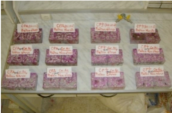
Figure 4: Demonstration of the carbonation fronts visualized following the spraying with phenolphthalein.
