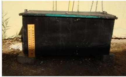
Figure 2. Steam Curing Chamber
